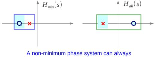
A non-minimum phase system can alway be decomposed into  $H_{min}(s) \cdot H_{all}(s)$
