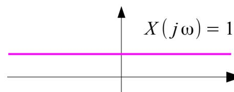
$$\begin{aligned} x(t) &= \frac{1}{2\pi} \int_{-\infty}^{+\infty} 2\pi\delta(\omega) e^{+j\omega t} d\omega \\ &= \int_{-\infty}^{+\infty} \delta(\omega) e^{+j\omega t} d\omega \\ &= \int_{-\infty}^{+\infty} \delta(\omega) d\omega = 1 \end{aligned}$$
