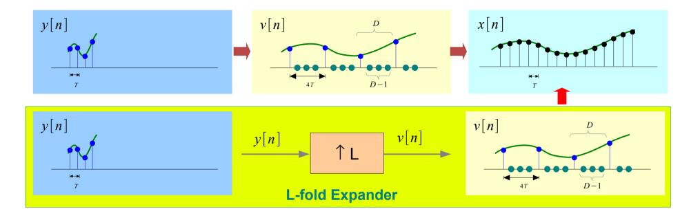
$$v[n] = S_L y[n] = \begin{cases} y[n/L] & \text{if mod}(n/L) = 0 \\ 0 & \text{L-fold Expander} \end{cases}$$
