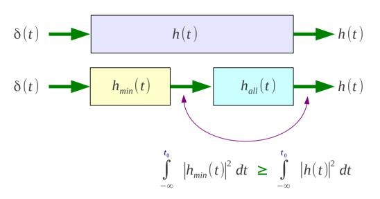
The signal energy until  $t_0$  of the minimum phase
