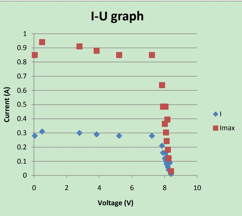
$$\left. \begin{array}{l} V_{P,\max} = 7,23 \text{ V} \\ I_{P,\max} = 0,85 \text{ A} \end{array} \right\} \text{Working point}$$
