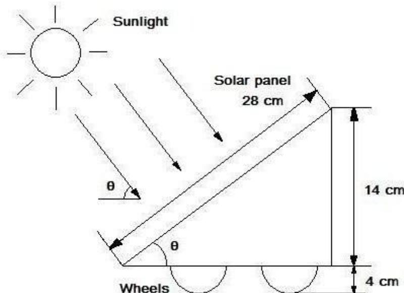
Maximum velocity at the maximum power:  $V = P_{\text{real}} / F_{\text{wheel}} = 4,31 / 1,36 = 3,17 \text{ m/s}$
