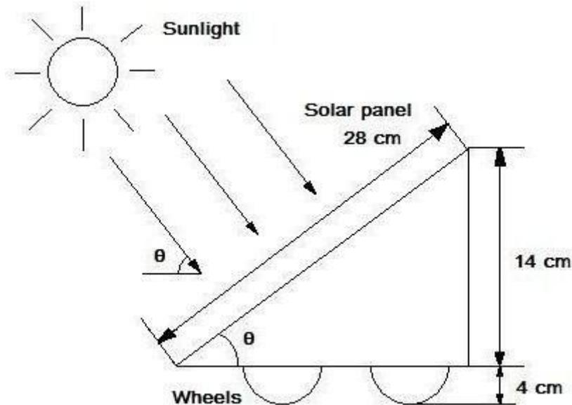
Maximum velocity at the maximum power:  $V = P_{\text{real}} / F_{\text{wheel}} = 4,31 / 1,19 = 3,62 \text{ m/s}$
