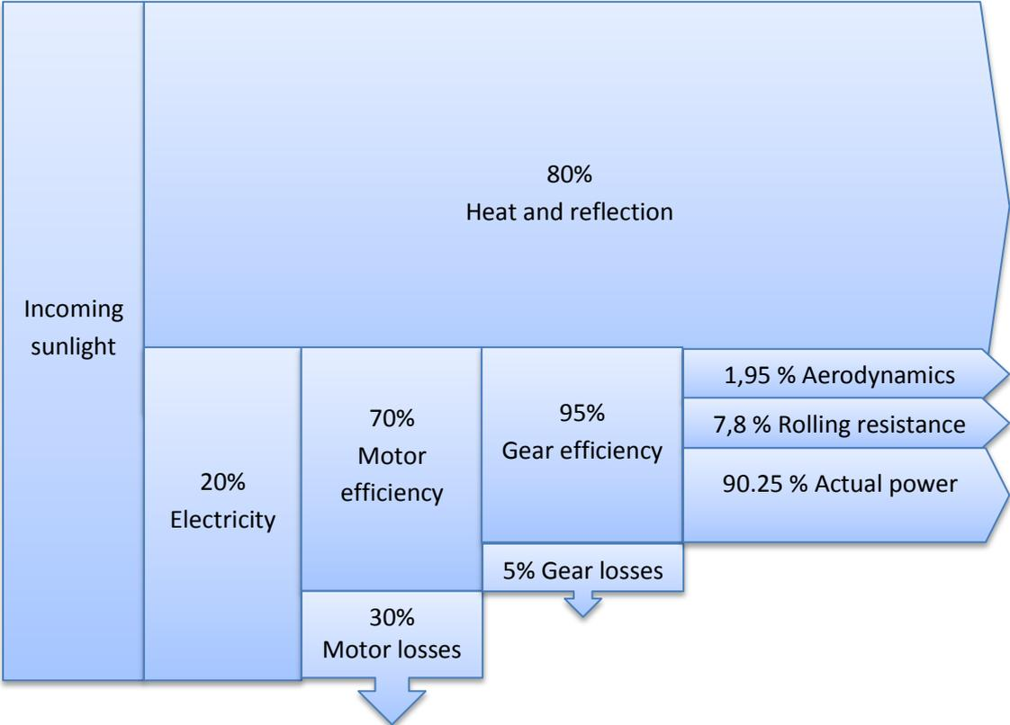
When we analyze this Sankey diagram, we can conclude that our car won't be very efficient. From the total energy that we get from the sun, there is only a small amount that we can use to drive our car. The actual power that you can see at the end of the Sankey diagram is no wasted energy. This is the energy that's left to move the wheels and let the car move.
