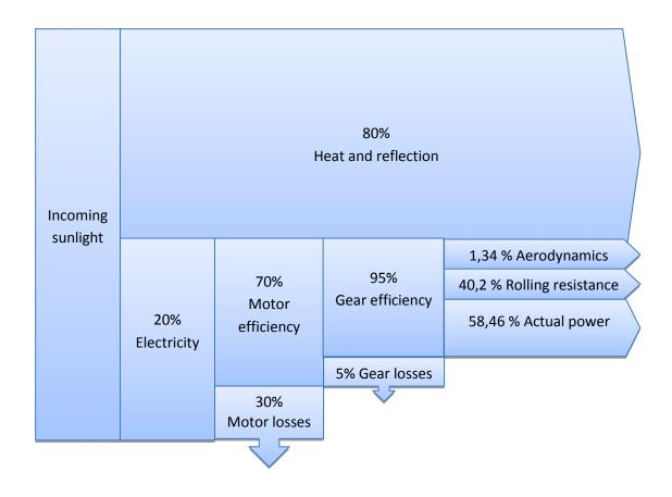
When we analyze the last three parts, we see that the aerodynamics is just a small loss of the total energy. Due to the rolling resistance, we almost lose the half of our energy. The energy that's left is used to move the car forward so we can call it the actual power of the car.
