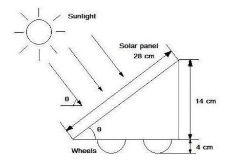
Maximum velocity at the maximum power: V =  $P_{real}$  /  $F_{wheel}$  = 4,31 / 1,36 = 3,17 m/s According to the formula, drag force:  $F_D$  = 0,5 \* 1,204 \* 0,09 \* 0,0316 \* 3,17<sup>2</sup>
