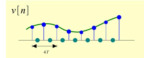
$$\begin{aligned}v[n] &= \frac{1}{2}x[n] + \frac{1}{2}e^{-j\pi n}x[n] \\ &= \frac{1}{2}e^{j\omega n} + \frac{1}{2}e^{-j\pi n}e^{j\omega n} \\ &= \frac{1}{2}e^{j\omega n} + \frac{1}{2}e^{+j(\omega-\pi)n}\end{aligned}$$
