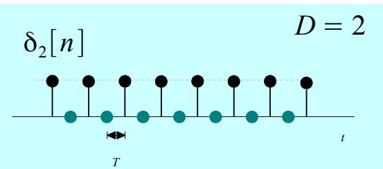
$$\begin{aligned}\delta_2[n] &= \frac{1}{2}(1 + (-1)^n) \\ &= \frac{1}{2}(1 + e^{-j\pi n}) \\ (e^{-j\pi} &= -1)\end{aligned}$$
