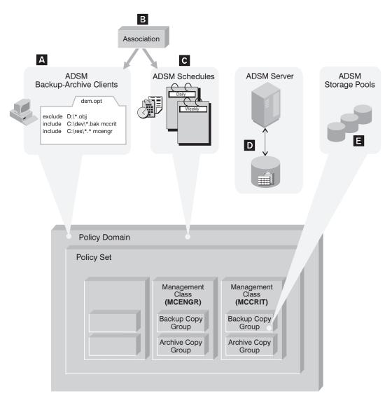
Figure 4. Automating Client Operations
