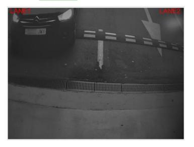
VIVOTEK ANPR will read the license plate and indicate on which lane the license plate was detected.
