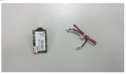
**Step 1.** Carefully pull out the damage SATADOM and its power cable. **Note:** be sure to power down the device before pulling out the SATADOM.
