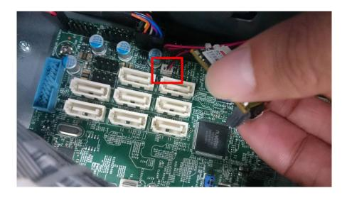
**Step 4.** Connect the SATADOM in the same slot as the damaged one. **Note:** connecting the SATADOM to different slots should not affect functionality, but we recommend installing in the same slot.
