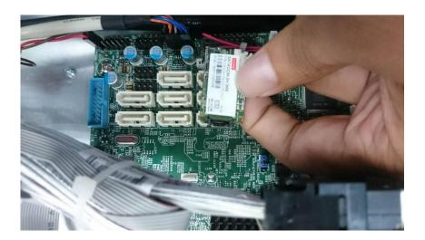
**Step 2.** Connect the power cable to the SATADOM to the board. (Power cable is included inside the packet send by RMA).
