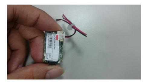
**Step 3.** Connect the power cable of the SATADOM to the board. (Power cable is included inside the packet send by RMA).
