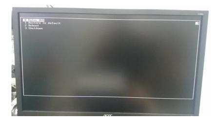
**Step 7.** Select Enter NVR and press "Enter". **Note:** this interface is normal, each time the NVR is initialized or restarted it will ask you to choose between these four options.
