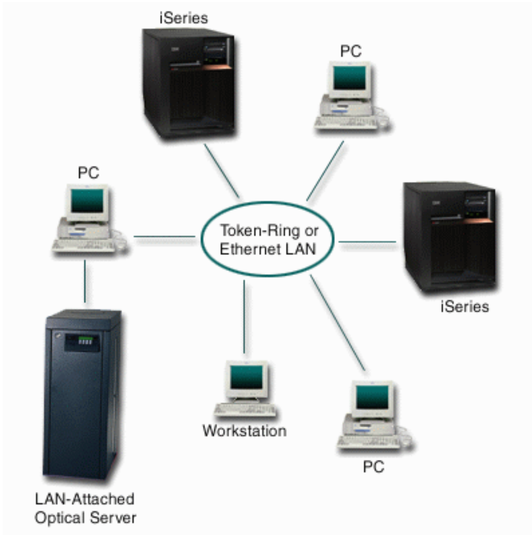
Figure 2. Example of Using iSeries servers with a LAN-Attached Optical Library
