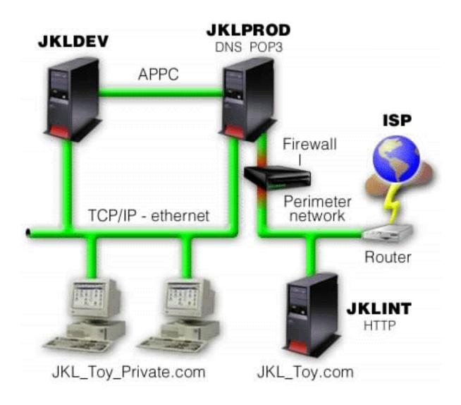
As shown in the diagram, JKL Toy company has two primary iSeries servers. They use one system for development (JKLDEV) and one for production (JKLPROD) applications. Both of these systems handle mission-critical data and applications. Consequently, they are not comfortable running their Internet applications on these systems. Instead, they have chosen to add a new iSeries server (JKLINT) to run these applications.
