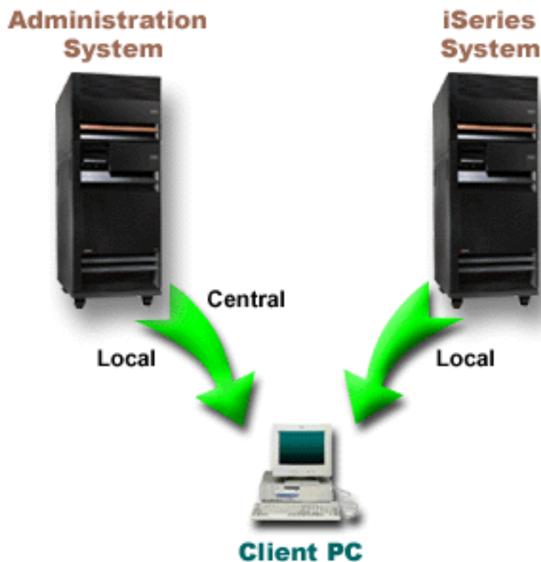
Figure 1. When a Client PC connects to a system, the Local Settings come from the system that you connect to. When you connect to an administration system, the Central Settings are sent to your Client PC from the administration system.
