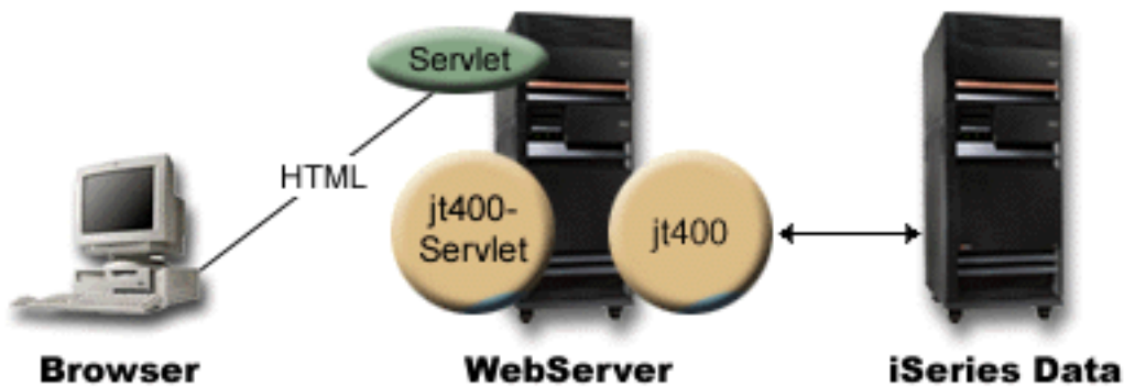
Figure 1: How servlets work
