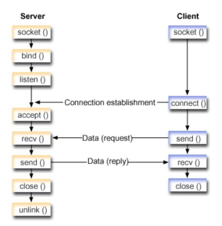
Socket flow of events: Server application that uses AF\_UNIX\_CCSID address family
