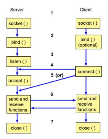
Typical flow of events for a connection-oriented socket:
