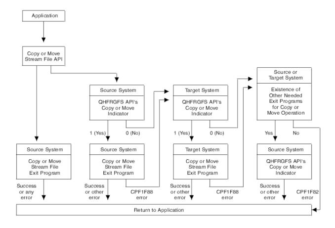
After determining that the file systems differ, the API tries to perform the copy operation in several different ways. If a method fails, the API proceeds to the next method. The possible methods are to call the following exit programs in the sequence listed:
