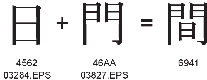
Figure 4. Combining two existing characters to make a UDC. Where 4562, 46AA, and 6941 are code points, and 03284 and 03827 are CID numbers.
