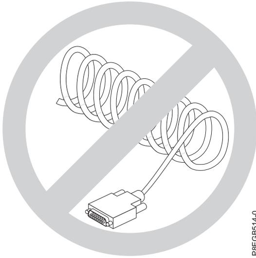
To minimize the electrical interference if you have excess video cable, arrange the cable in figure-eight loops, as shown in the following illustration. Secure the cable in the middle with a cable tie or strap.
