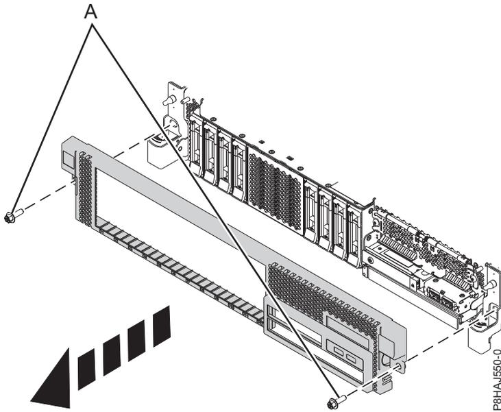
Figure 5. Removing the front cover
