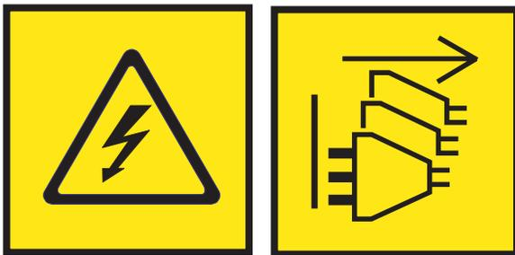
**DANGER:** Multiple power cords. The product might be equipped with multiple AC power cords or multiple DC power cables. To remove all hazardous voltages, disconnect all power cords and power cables. (L003)
