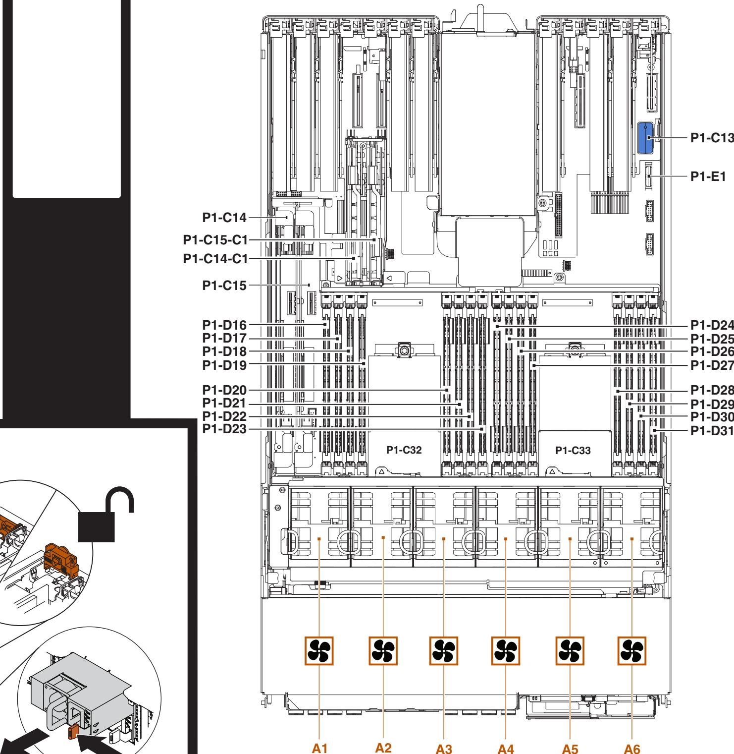
**Terra Cotta** on the part indicates the system may not be required to be powered off to perform service. This is dependant on the system configuration and preparatory steps may be required before the service action is taken on the system.
