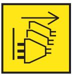
**DANGER:** Multiple power cords. The product might be equipped with multiple AC power cords or multiple DC power cables. To remove all hazardous voltages, disconnect all power cords and power cables. (L003)
