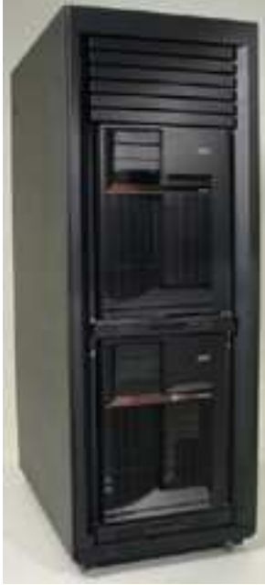
Figure 14. 0551 model 9406-270 Rack system units
