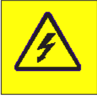
Figure 10 Hazardous Voltage, Current, or Energy
