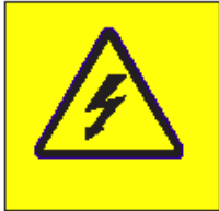
Figure 12 Hazardous Voltage, Current, or Energy
