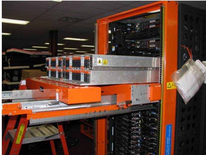
Figure 42 DE slid out slowly to point of latch engagement
