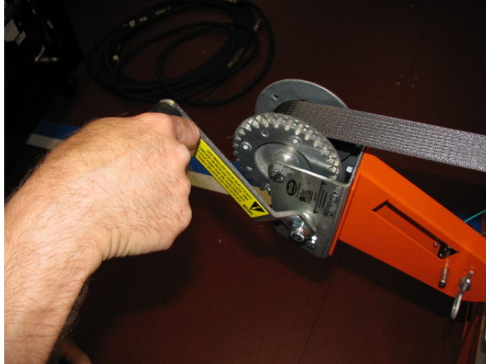
Figure 55 Use Winch to pull DE onto transfer cart
