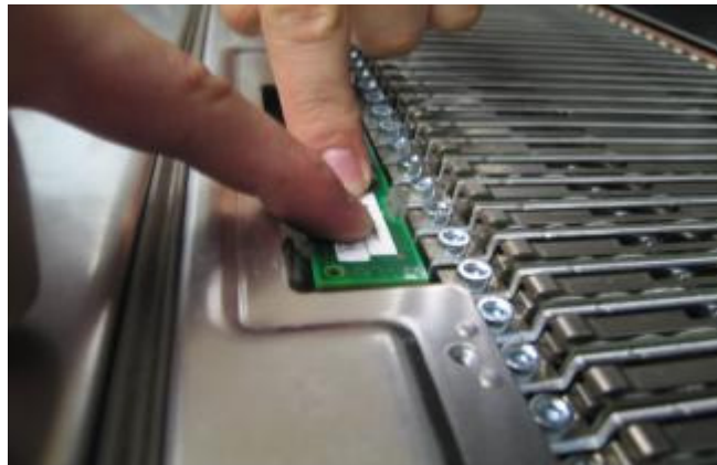
Figure 31 Replacing VPD card Continued
