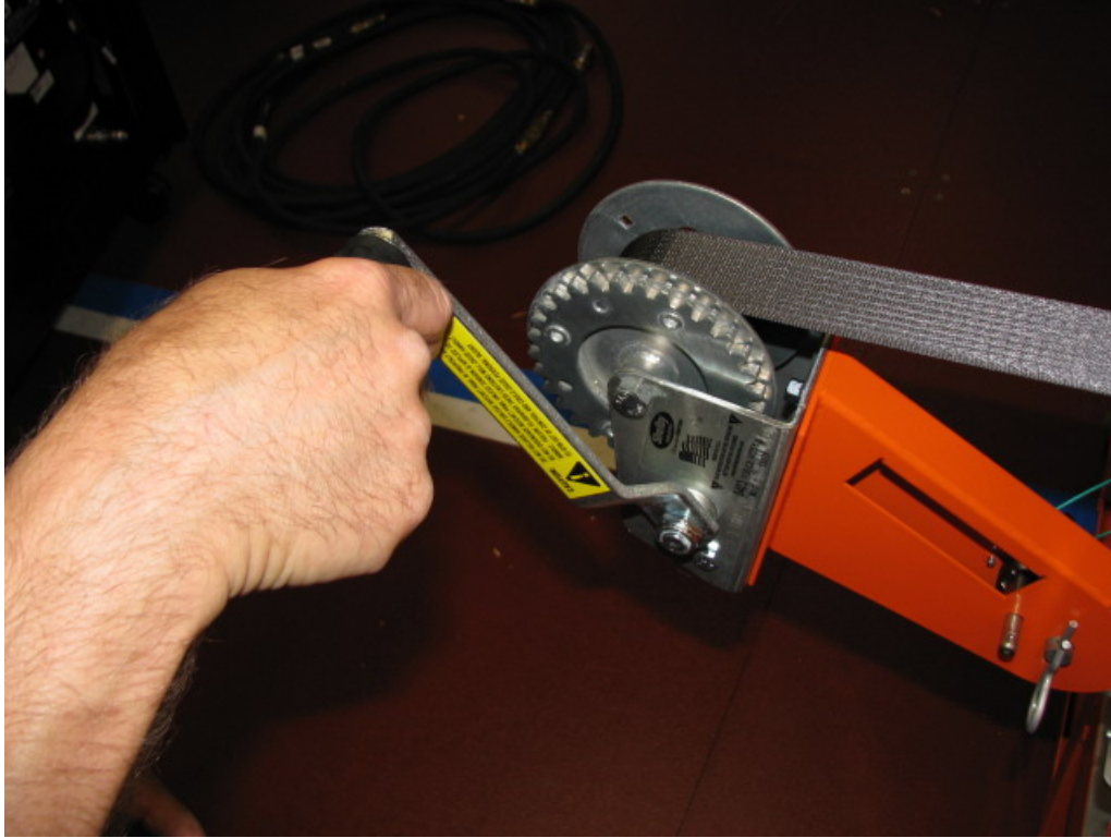
Figure 46 Use winch to pull BPE onto transfer cart
