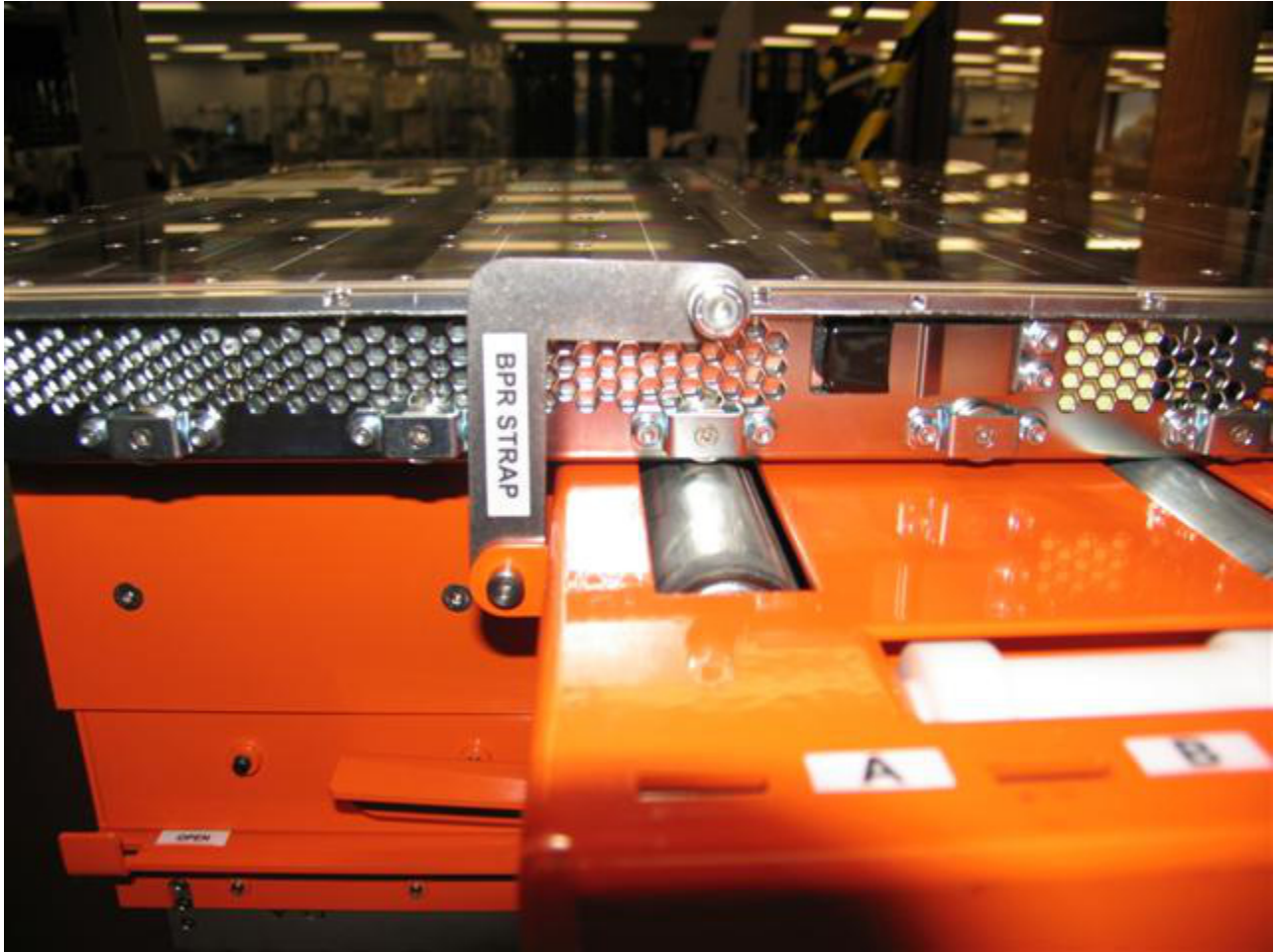
Figure 32 BPR Safety Strap Attached to BPR (similar for BPD also)
