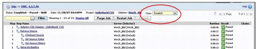
Figure 3: Sample screen shot showing where the class property can be changed for a run
