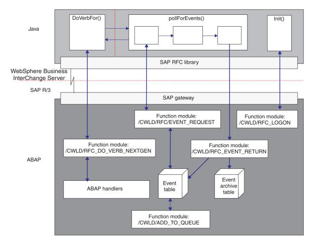
Figure 5. ABAP Extension Module architecture
