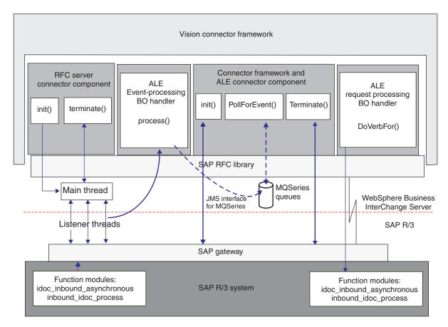
Figure 17. ALE Module architecture
