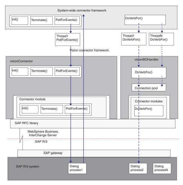
Figure 3. Multi-Threading architecture of the connector for SAP
