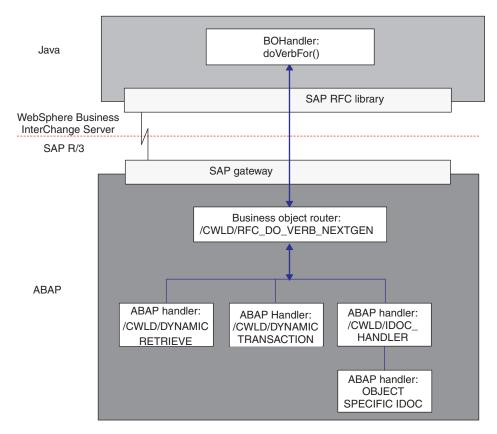
Figure 7. Adapter-provided business object processing components
