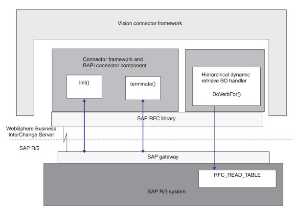
Figure 30. Hierarchical Dynamic Retrieve Module architecture
