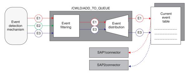
Figure 11. Event priority with function module /CWLD/ADD\_TO\_QUEUE
