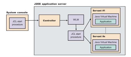
Within each server are two kinds of address spaces: controllers and servants. A controller runs system authorized programs and manages tasks, such as communication, for the server. Each server has one controller that you start with a JCL start procedure when you enter the appropriate start command on the MVS console.
