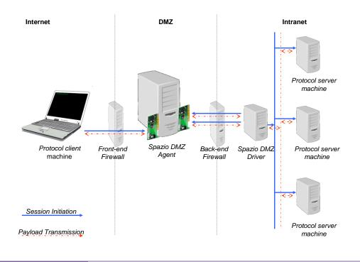
The firewall proxy means that parties beyond the external firewall can only ever initiate sessions with the proxy, which is situated in the DMZ (between the Enterprise's internal firewall layer and external firewall layer). Furthermore, data is never stored in the DMZ; it is always transient.
