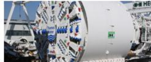
120-metre-long Lee Tunnel boring machine
