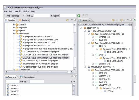
CICSACB7 shows the added ENQ/DEQ running on the L8 TCB since it is defined as threadsafe and EWHWORKP issues a DB2 select which puts the work over on the L8 TCB.
