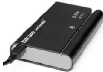
nonClonable™ Swipe reader for authenticating blister packs
