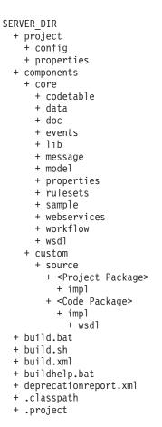
Figure 1. Cúram Application Structure
