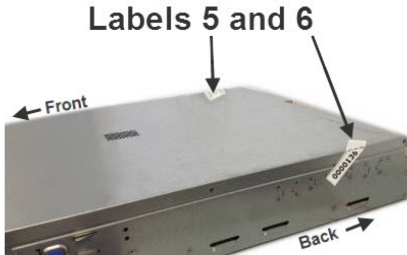
Figure 1-4 Labels 5 and 6 applied across the upper-left and upper-right side of the appliance.
