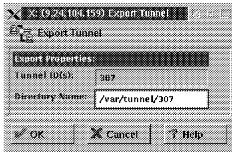
Figure 117. Exporting the Tunnel Definition
