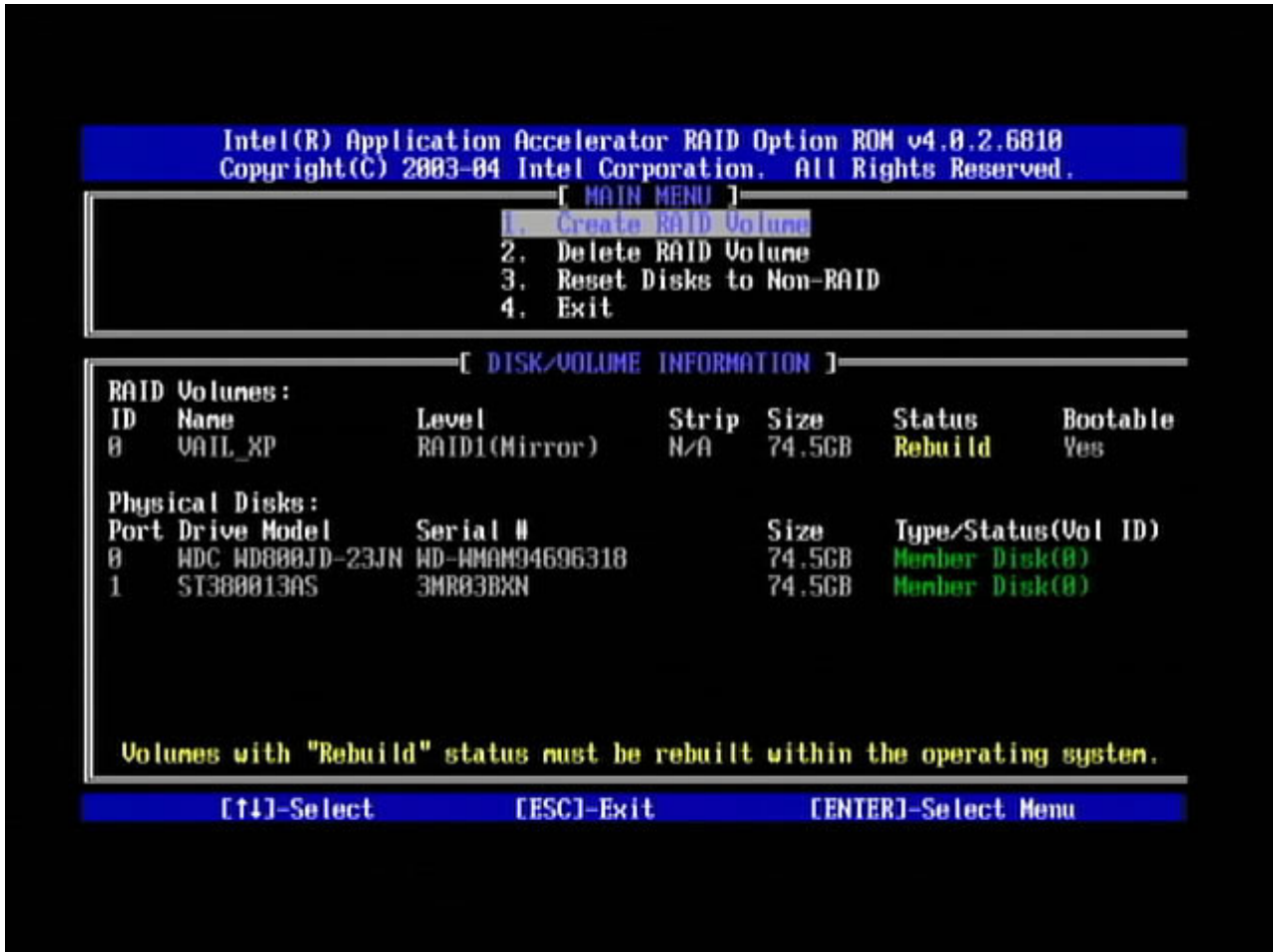
Figure 4. Example of the RAID setup menu
