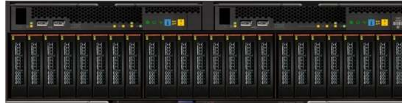
IBM V7000 Storage Node
