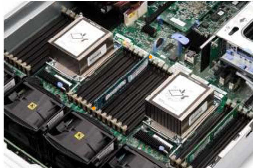
Light Path Diagnostics Component Level Lights Indicates what individual component has PFA alert or has failed
