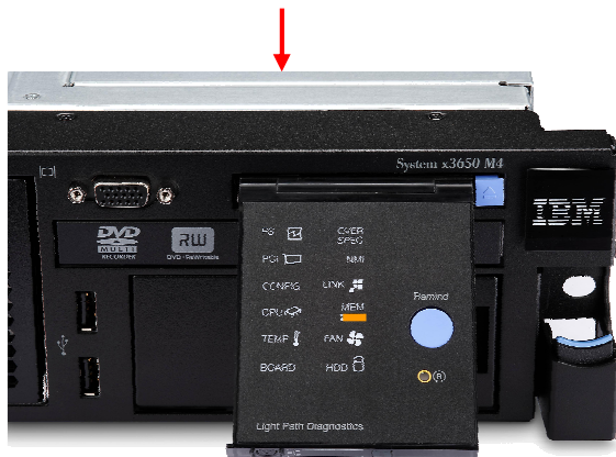
Pop-Out Light Path Diagnostics Panel Indicates what subsystem has problem
