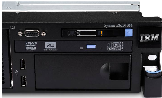
Front of Light Path Diagnostics Panel Amber light indicates there is a problem with the server
