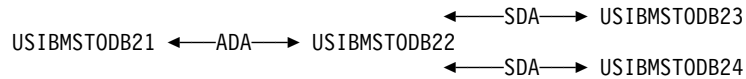
Figure 72. Example of a DB2 transaction involving four sites. ADA refers to DRDA access, SDA to DB2 private protocol access
