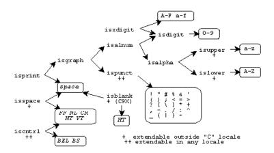
The diagram tells you that the function is print (page 57) returns nonzero for space or for any character for which the function isgraph (page 57) returns nonzero. The function isgraph, in turn, returns nonzero for any character for which either the function isalnum or the function ispunct returns nonzero. The function isdigit, on the other hand, returns nonzero only for the digits 0-9.
