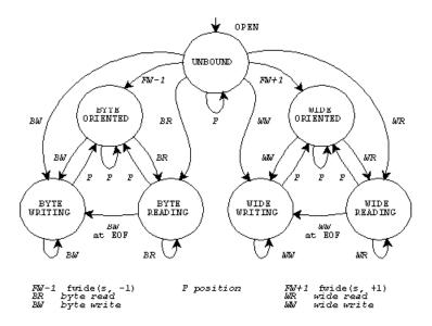
Each of the circles denotes a stable state. Each of the lines denotes a transition that can occur as the result of a function call that operates on the stream. Five groups of functions can cause state transitions.
