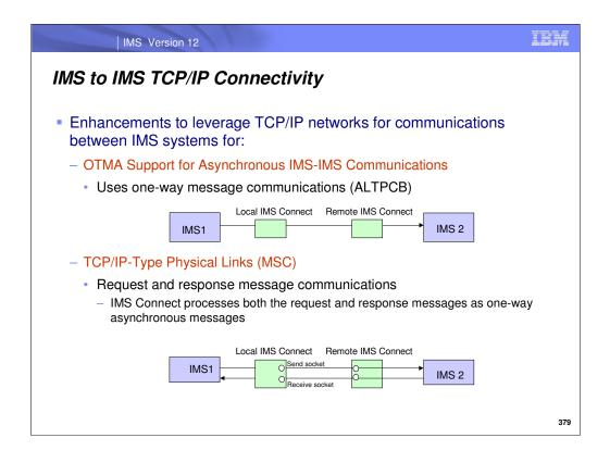
IMS version 12 provides the ability to send messages from a local IMS to a remote IMS over a TCP/IP network. The messages are sent over the TCP/IP network by a local IMS Connect and received by a remote IMS Connect. The local IMS communicates with the local IMS Connect and the remote IMS communicates with the remote IMS Connect. IMS can send messages using OTMA or MSC protocols.
