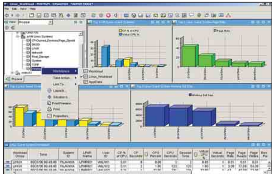
Tivoli OMEGAMON XE on z/VM and Linux workspaces help you easily investigate problems related to z/VM and Linux performance, with views of metrics including CPU consumption (guest/virtual and z/VM overhead), paging rates, total page reads (and writes) and working set size.
