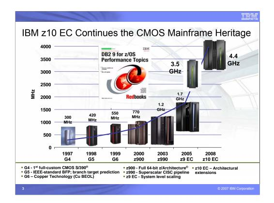
The design of the IBM System z10<sup>™</sup> processor chip is the most extensive redesign in over 10 years, resulting in an increase in frequency from 1.7 GHz (z9 EC) to 4.4 GHz on the z10 EC. The z10 BC processors run at 3.5 GHz.
