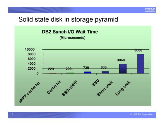
Understanding where solid state disk fits into the storage hierarchy is very important. This device is very fast for random IO, but it's more expensive than magnetic disk.
