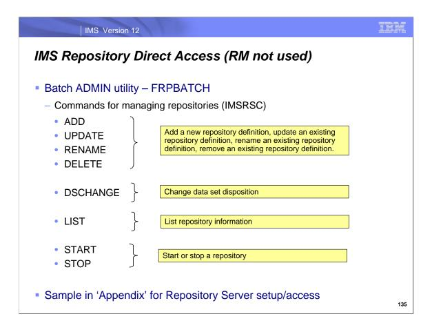
A repository batch ADMIN utility (FRPBATCH) is provided to help manage IMSRSC repositories. There are 8 commands provided. This utility does not use RM to access the repository; rather it accesses the repository directly as a batch job using XCF. This information about IMSRSC repositories is kept in the catalog repository.
