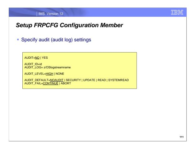
The audit parameters determine if the audit log exists and what information it contains. The audit levels listed in the AUDIT\_DEFAULT keyword create an increasing number of audit log entries. SYSTEMREAD will create the most and is the highest level of auditing.
