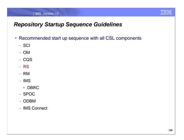
The repository server address space must be up before RM comes up (RM initialization PROCLIB member CSLRIxxx with REPOSITORY section). Then IMS can come up (uses DFSDFxxx PROCLIB member sections). If IMS comes up before RM with RM not enabled for a repository, IMS will abend with a U400.
