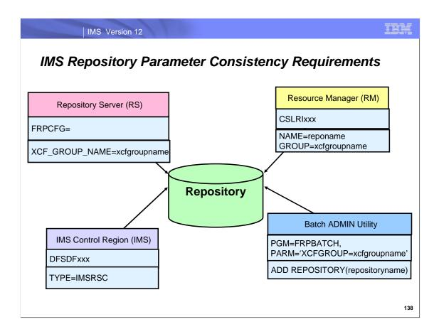
This diagram depicts the parameter settings needed by Repository Server (RS), the Resource Manager (RM), the IMS Control Region (IMS), and the Batch ADMIN Utility that must be identical for access to a particular repository.
