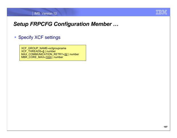
The XCF groupname must be specified; this groupname will be used for communications between the RS address space and the RM address space(s).
