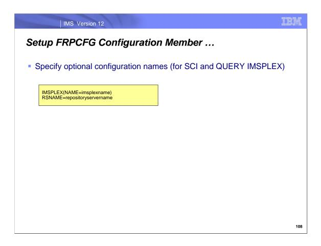
The IMSPLEX and RSNAME parameters are used to indicate that the RS should register with SCI, so that the repository server will be included as an address space in the output of a QUERY IMSPLEX command.
