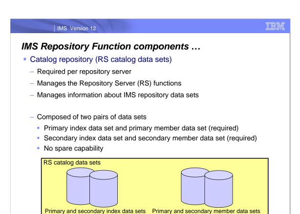
The catalog repository data sets (RS catalog data sets) are used by the repository server itself to store its own data. These are required per repository server and must be allocated before a repository server can start up.
