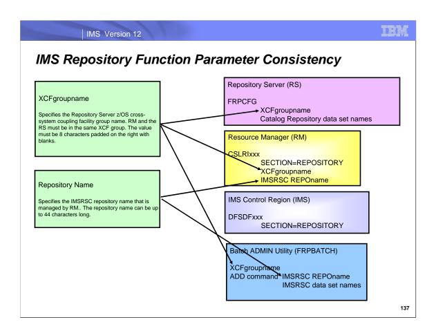
There are two major 'naming' parameters that tie together all the processing for a repository server. The first is the z/OS XCFgroupname, which is used for communications to the repository server. The same XCFgroupname must be used in all the member definitions that use a particular repository. The second is the name of the IMSRSC repository which holds the DRD definitions for the IMSplex.
