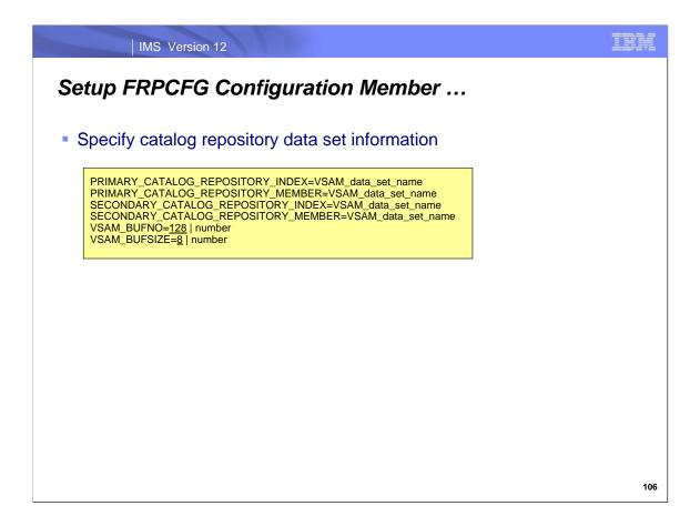
For the catalog repository data sets, you must specify the names for the primary catalog repository index data set, the primary catalog repository member data set, and the names of their secondary copies. The repository server uses VSAM LSR for buffering using an 8K buffer size.
