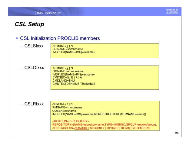
CSL initialization PROCLIB members must be set up when using the repository server. The SCI initialization member (CSLSIxxx) and the OM initialization member (CSLOMxxx) just need to contain standard CSL parameters (in black).
