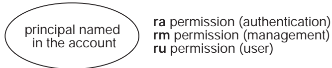
Figure 73. Permissions Required to Change Management, Authentication, and User Information (Except Passwords) For Accounts
