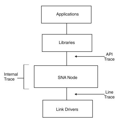
Figure 1. Tracing Interfaces
