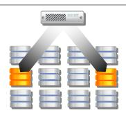
For ultra-high availability applications, synchronously mirror application data between two separate disk enclosures attached to the same Storwize V7000 system.
